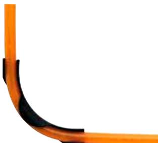
Schlüter-BEKOTEC-THERM-ZW is an angle clip of synthetic material for defined 90° bends of the heating pipes in diameters 10, 12, 14 or 16 mm in the distributor cabinet. The angle clip is easy to attach to the heating pipes from the side. The use of the clips is recommended to facilitate installation in the distributor cabinet if the thickness of the screed layer is relatively low.
