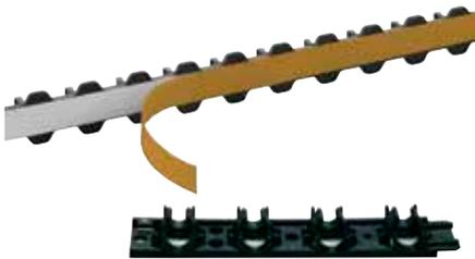
Schlüter-BEKOTEC-ZRKL is a pipe clamping strip for securing the pipes on the levelling panel. The self-adhesive clamping strips are simply adhered to the levelling panels in front of the heating circuit distributor.
