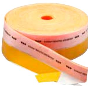
Schlüter-BEKOTEC-BRS/KSF is an edging strip of closed cell polyethylene foam with an integrated foil leg that features an adhesive strip on both sides for attachment. The edging strip is pressed toward the wall by the adhesion on the substrate and the pre-tensioning of the integrated foil leg. When the studded panel BEKOTEC is laid on top of the adhesive strip, flowing screed can no longer flow underneath the panel.
