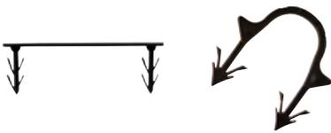
Schlüter-BEKOTEC-THERM-RH are plastic clips with barbs for anchoring 16 mm heating pipes into the BEKOTEC studded panels in critical areas. Size 75 is suitable for multiple heating pipes, while size 17 only accommodates a single pipe.
