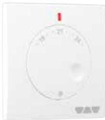
Schlüter-BEKOTEC-THERM-ER is a wired thermostat for heating/cooling. The setpoint can be set from 8 to 30 °C (with restrictions if necessary) and is transmitted to the connection module EAR 2/6 with a cable (DC 5 V, SELV). The "Control" base model provides the voltage. The operating state "heating/cooling" is displayed by the "red/blue" colour change in an LED.
