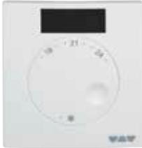
Schlüter-BEKOTEC-THERM-ER/WL is a remote-controlled thermostat for heating/cooling. The setpoint can be set from 8 to 30 °C (with restrictions if necessary) and is wirelessly transmitted to the connection module EAR 2/6 WL. The EET timer unit manages the temperature reduction. The energy supply consists of an integrated solar cell, or alternatively with a supplied button cell.
