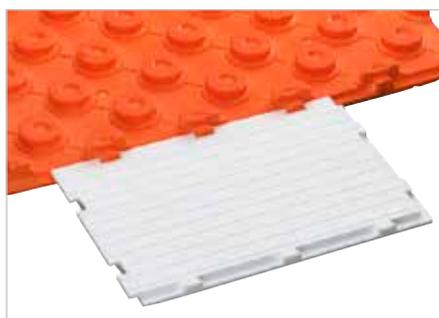
Schlüter-BEKOTEC-ENR is a levelling panel to reduce cutting waste in edge areas and transitions (e.g. doors, niches), for areas in which no heating pipes are installed. It can also be used in front of heating circuit distributors to facilitate heating pipe installation.
