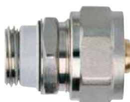
Schlüter-BEKOTEC-THERM-AN is a connector fitting made of nickel plated brass. One side has a self sealing 1/2" (DN 15) external thread, while the other side features a 3/4" (DN 20) compression fitting for connecting the 14 mm or 16 mm Schlüter heating pipe – fits all Euro cone fittings.
