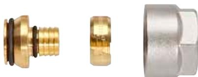
Schlüter-BEKOTEC-THERM-KV is a clamping ring for the hot and cold leg made of nickel plated brass. It connects the Schlüter heating pipes (diameter 10, 12, 14, 16 mm) with the Schlüter heating circuit distributor.
