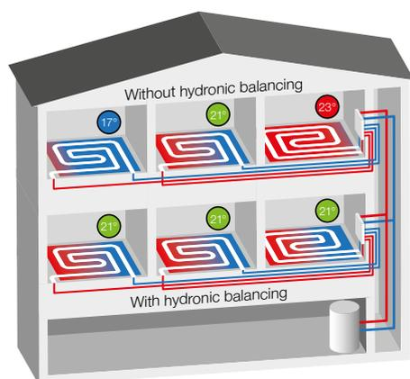
Hydronic balancing drives the energy efficiency of heating and cooling systems. Since every heating circuit receives exactly the right supply volume, the heating system is especially responsive and energy efficient. Intelligent adaptive balancing can optimise the heat distribution even further than static adjustment. It offers the following advantages:
