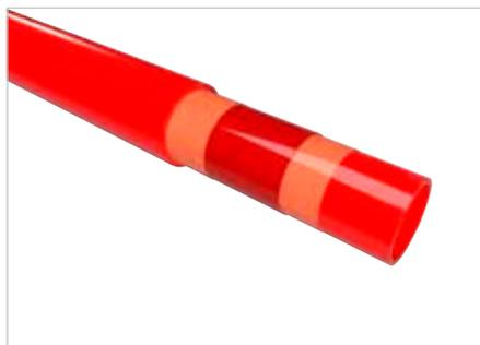
Schlüter-BEKOTEC-THERM-HR is a 5-ply bonded heating pipe made of a high-quality polymer material (PE-RT) with an oxygen diffusion barrier in the centre. The highly flexible heating pipe, which complies with DIN 16833, is optimised for installation in BEKOTEC system panels. Its oxygen tightness is certified according to DIN 4726, and the product is subject to continuous quality monitoring.
