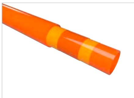
Schlüter-BEKOTEC-THERM-HR is a 5-ply bonded heating pipe made of a high-quality polymer material (PE-RT) with an oxygen diffusion barrier in the centre. The highly flexible heating pipe, which complies with DIN 16833, is optimised for installation in BEKOTEC system panels. Its oxygen tightness is certified according to DIN 4726, and the product is subject to continuous quality monitoring.
