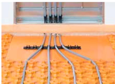
The levelling panel Schlüter-BEKOTEC-ENFG is installed in front of heating circuit distributors to simplify the heating pipe installation in the distributor cabinet. The polystyrene panel is adhered to the studded panel with the supplied double sided adhesive tape (6 m).
