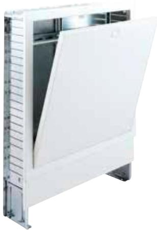
Schlüter-BEKOTEC-THERM-VSE is a distributor cabinet for concealed mounting to house the Schlüter heating circuit distributor manifold and the matching control components. The concealed cabinet consists of fully galvanised steel with perforations in the lateral walls for inserting the connector pipes. The front side (door and frame) is powder coated.
