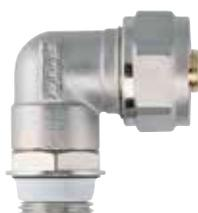
Schlüter-BEKOTEC-THERM-AW is an angled connection fitting made of nickel plated brass that can be rotated. One side has a self sealing 1/2" (DN 15) external thread, while the other side features a 3/4" (DN 20) compression fitting for connecting the 14 mm or 16 mm Schlüter heating pipe.
