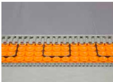
Schlüter-DITRA-HEAT is a polypropylene membrane with a cut back stud structure and an anchoring fleece laminated on the underside. It is a universal substrate for tile coverings, which serves as an uncoupling layer, bonded waterproofing and vapour barrier, designed for the attachment of the matching heating cables for floor and wall heating solution.
