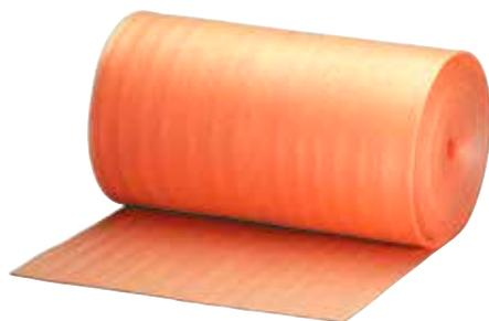
Schlüter-BEKOTEC-BTS is a 5 mm insulation layer of closed cell polyethylene foam for installation below the studded screed panels Schlüter-BEKOTEC-EN-P, -EN-PF and -EN 23 F. The use of BEKOTEC-BTS results in a significant improvement of sound insulation. The material can be used if the required construction height is not sufficient for a thick insulation layer of polystyrene or mineral fibre. The maximum floor load must be limited to 2 kN/m<sup>2</sup>.
