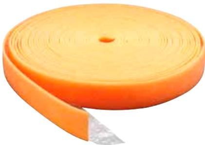
Schlüter-BEKOTEC-BRS is an edging strip of closed cell polyethylene foam with an integrated foil leg. The edging strip is installed along walls or fixed room components. The foil leg is installed beneath the Schlüter-BEKOTEC panels or the PE foil cover and is suitable for conventional cement screeds. The finishing strip Schlüter-BEKOTEC-BRSK is equipped with an additional adhesive strip for attachment to the wall.
