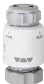
Schlüter-BEKOTEC-THERM-ESA is an actuator for operation with 230 Volt to control the flow of the cold leg valves. It is mounted on the valves of the Schlüter heating circuit distributor cold leg with screws (M30 x 1.5), design according to IP54 (splash water protection).
