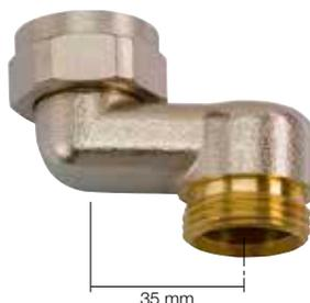
Schlüter-BEKOTEC-THERM-S35 is an offset connector made of nickel plated brass that features a 3/4" (DN 20) cone joint nut on one side and a 3/4" (DN 20) cone connector thread on the other side for connecting the Schlüter heating pipes with diameters of 10, 12, 14 or 16 mm.
